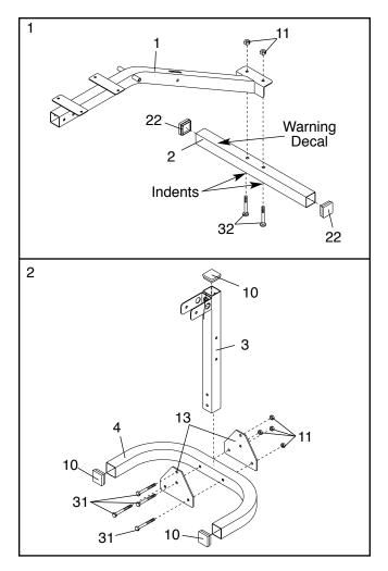
3. Attach the Front Leg (3) to the Bench Frame (1) using two Joint Plates (12), four M10 x 70mm Bolts (31), and four M10 Nylon Locknuts (11).
